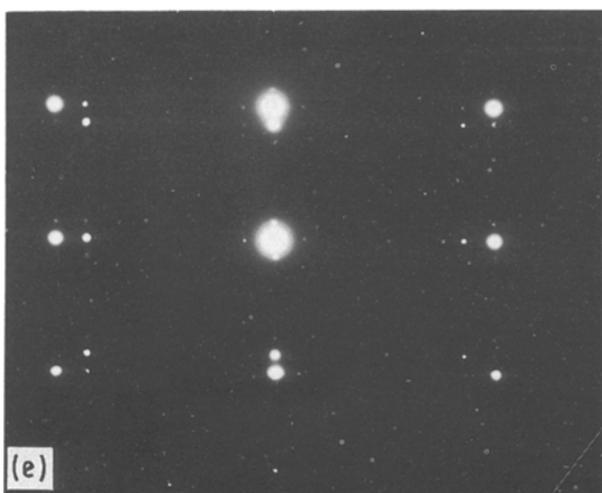
Figure 7 (a, b) BF transmission electron micrographs of CrN lamellae in twinned austenite of 1.0 N (wt %) material. (c) SADP and (d) corresponding schematic diagram from twinned austenite/CrN region. (e) SADP [112] zone axis (austenite matrix outside bright spots, inside spots are from CrN and double diffraction) from CrN/austenite.
